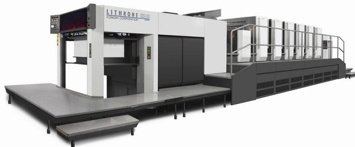
GLX-640+C(Six-color Print Quality Assessment System[PQA-S]-equipped 40-inch offset printing press with inline coater)
